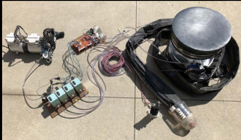
A growing soft robot, Sadie worked with at Stanford
