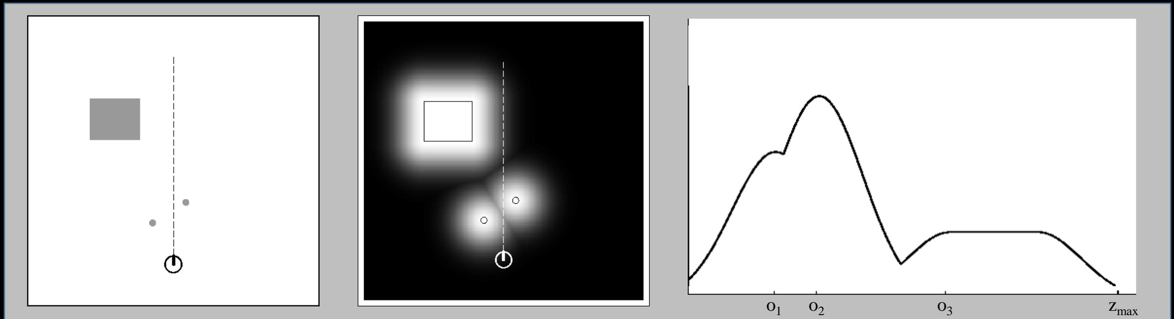
(a) Example environment with three obstacles (gray), Robot takes a measurement  $z_k^t$  (dashed line)
