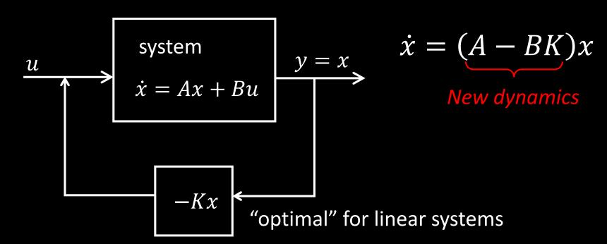
A linear controller (K matrix) can be optimal for linear systems!
