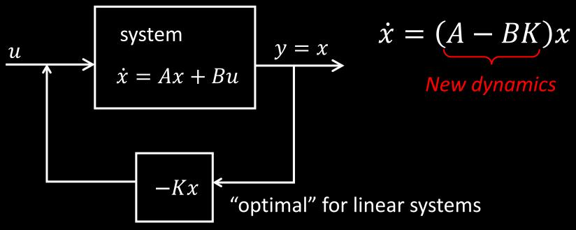
$$\underline{\dot{x}} = \underline{\underline{Ax}} + \underline{\underline{Bu}}$$
