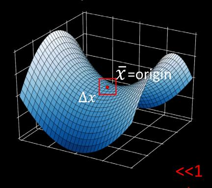
$$\dot{x} = f(\bar{x}) + \frac{Df}{Dx}|_{\bar{x}}(x - \bar{x}) + \frac{D^2f}{D^2x}|_{\bar{x}}(x - \bar{x})^2 + \frac{D^3f}{D^3x}|_{\bar{x}}(x - \bar{x})^3 + \cdots$$
