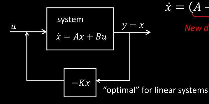
$$\underline{\dot{x}} = \underline{\underline{Ax}} + \underline{\underline{Bu}}$$
