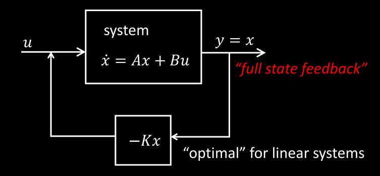
$$\underline{\dot{x}} = \underline{\underline{Ax}} + \underline{\underline{Bu}}$$
