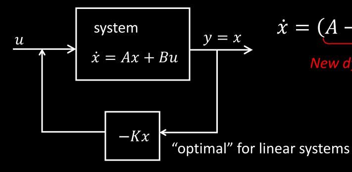
$$\underline{\dot{x}} = \underline{\underline{Ax}} + \underline{\underline{Bu}}$$
