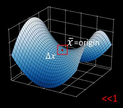
$$\dot{x} = f(\bar{x}) + \frac{Df}{Dx}|_{\bar{x}}(x - \bar{x}) + \frac{D^2f}{D^2x}|_{\bar{x}}(x - \bar{x})^2 + \frac{D^3f}{D^3x}|_{\bar{x}}(x - \bar{x})^3 + \cdots$$
