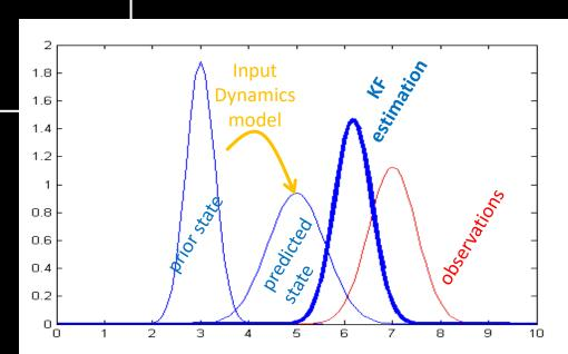
State estimate:  $\mu$ (t) State uncertainty:  $\Sigma$ (t) Process noise:  $\Sigma_u$ Kalman filter gain:  $K_{KF}$ Measurement noise:  $\Sigma_z$
